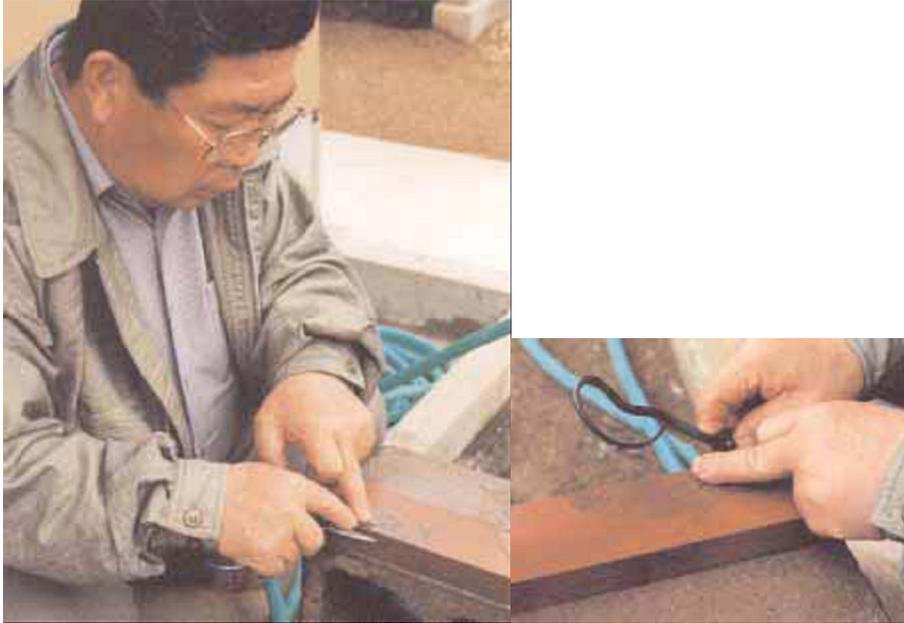
Mr. Mitsuya maintains his shears with water stones that he keeps in a small water-filled urn. If the edges of the blades are in pretty good condition, he uses a 1,000 grit stone for sharpening and a natural cut stone (like one of our "Washita" stones) for polishing. Before sharpening, he "dresses" or grinds flat each side of the sharpening stone by rubbing it firmly against a concrete block.
