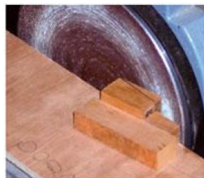
3. Cut the tapers on each leg by hand or on a bandsaw, or sand away the excess as shown here.
