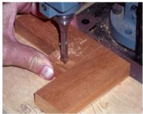
2. Make a simple L-shaped jig to keep your mortises consistent.
